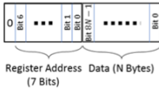
Figure A1-4: LoRaWAN Port 100 Read Response Format
