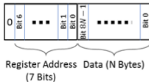
Figure 3-1: Bit Indexing Scheme for Configuration Registers
