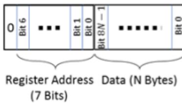
Figure 3-3: Bit Indexing Scheme for Configuration Registers
