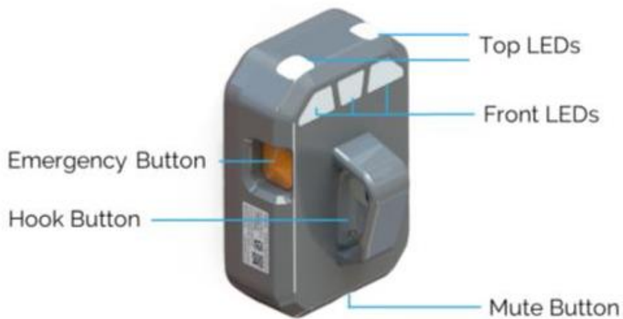
Figure 5-3: External User Interfaces on SEAL/SEAL Ex Clip variant
