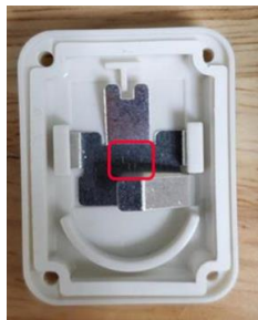
Figure 2-3: Polarity Marker and Battery Insertion
