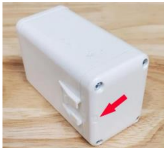
Figure 2-4: Proper Replacement Orientation of the Battery Cover
