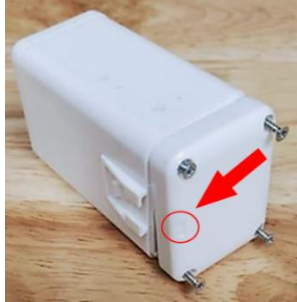
Figure 2-2: Removing the Battery Cover Screws
