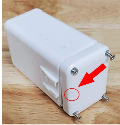
Figure 2-6 Removing the Battery Cover Screws
