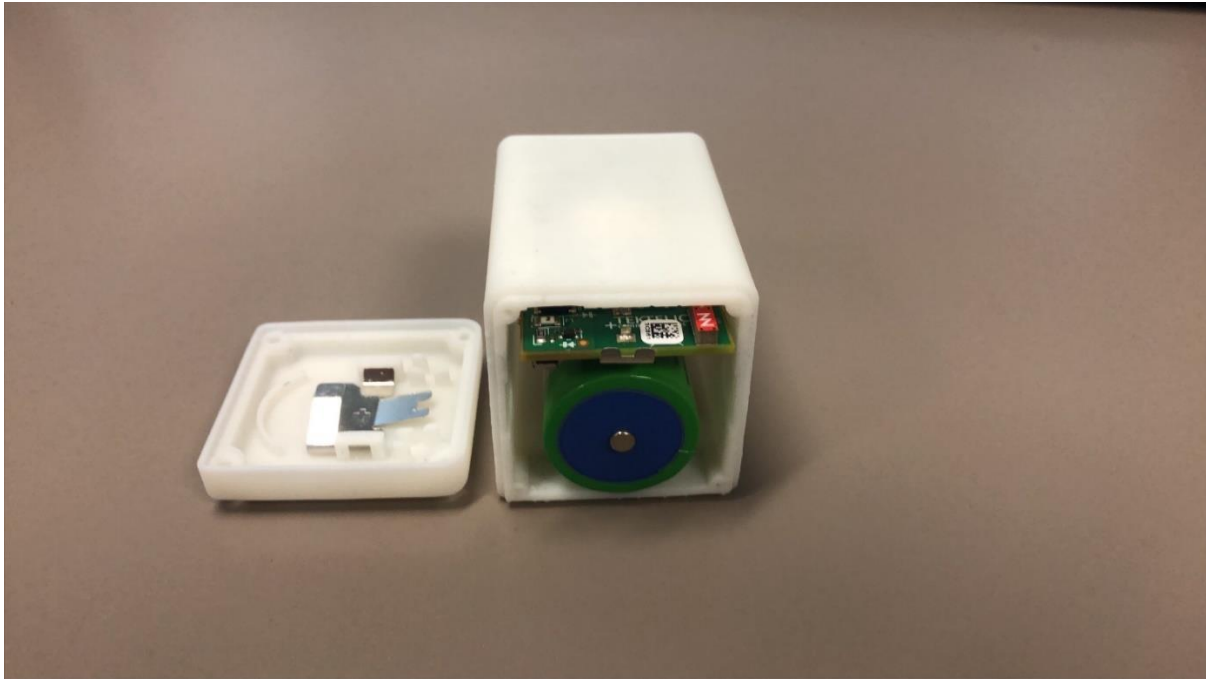
Figure 1-4: Battery Polarity Markers and Insertion
