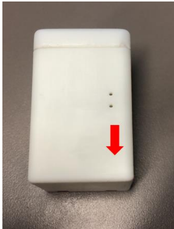
Figure 1-1: Sensor’s front view showing the location for applying magnetic pattern
