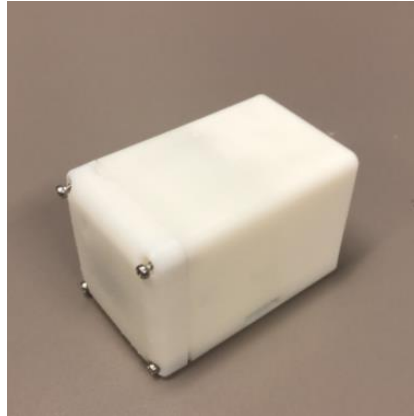
Figure 1-3: Removing the Battery Cover Screws
