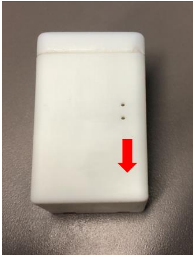
Figure 2-6: Magnetic Reed Switch Location
