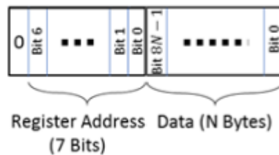
Figure 4-1: Bit Indexing Scheme for Configuration Registers
