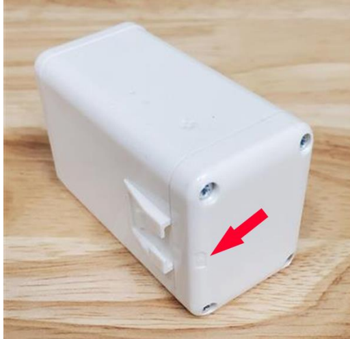
Figure 2-11: Proper Replacement Orientation of the Battery Cover
