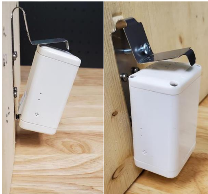
Figure 2-3: Attaching the Sensor to the Mounting Bracket
