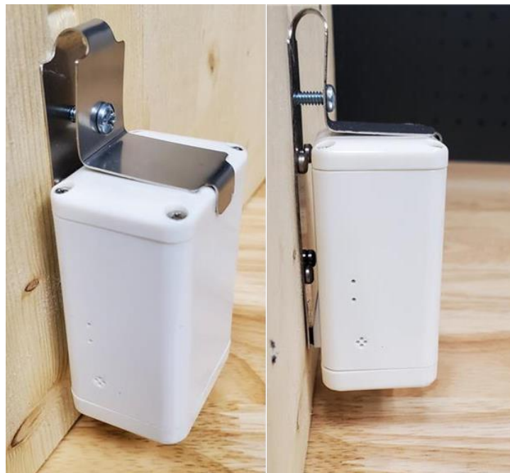
Figure 2-4: Securing the Sensor in the Mounting Bracket with a Fifth Screw
