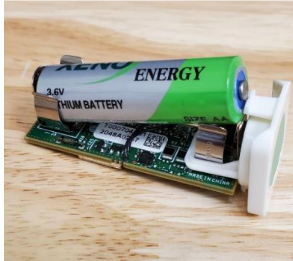
Figure 2-6: Battery Polarity Orientation
