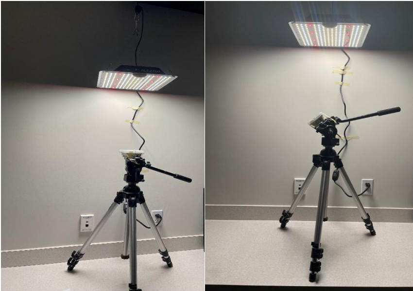
Figure 1: Test Setup – Left picture: Sensor at 0°, Right Picture: Sensor at 45°
