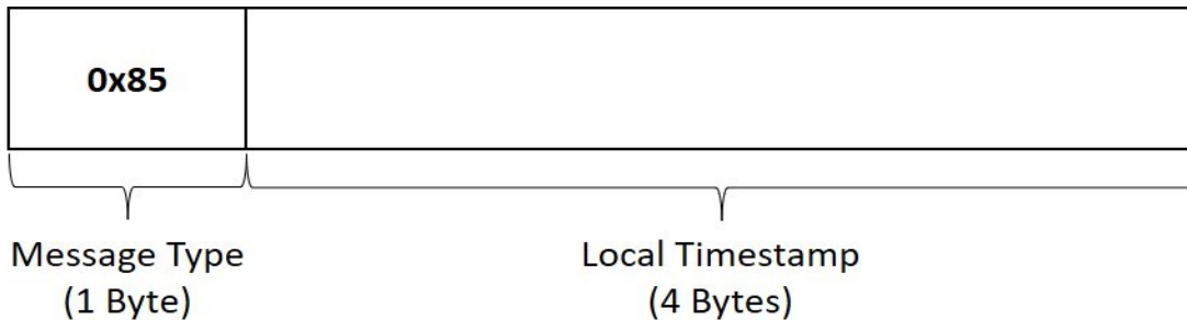
Figure 3-2: Frame format of sensor timestamp response in an UL payload.
