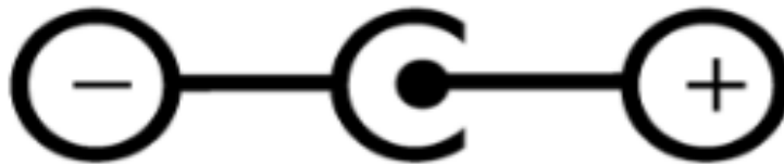
Figure 5: DC Power Connection Polarity
