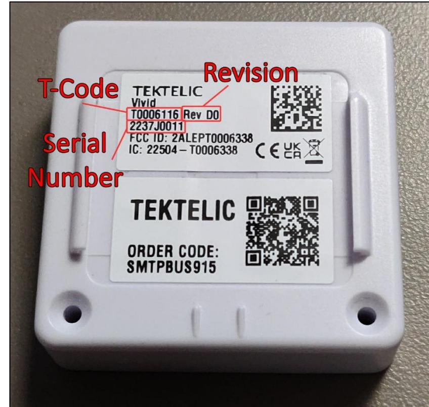
Figure-1 Sensor Identification
